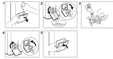
13.10 Cleaning the inlet hose and the valve filter
