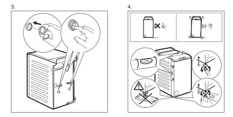
Adjust the appliance correctly to prevent vibration, noise and movement of the appliance when it operates.
