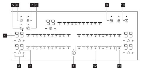
Use the sensor fields to operate the appliance. The displays, indicators and sounds tell which functions operate.
