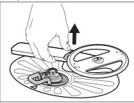
Wash the spray arm under running water. Use a thin pointed tool, e.g. a toothpick, to remove particles of soil from the holes.
