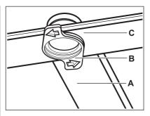
Release the stoppers on the sides of the sliding rails of the cutlery drawer and pull the drawer out.
